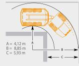
Turning radius according to ISO 7457: 8.42 m
